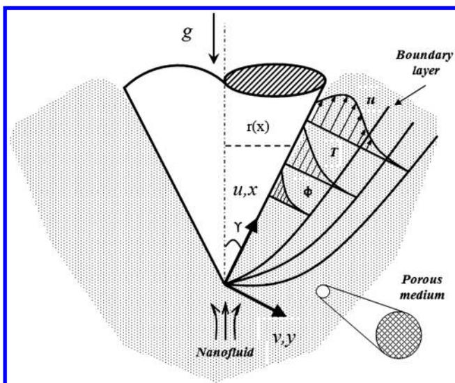
Fig. 1 The physical model and the coordinate systems used to model convective heat transfer around a vertical cone embedded inside a homogeneous porous media saturated with a nanofluid.
