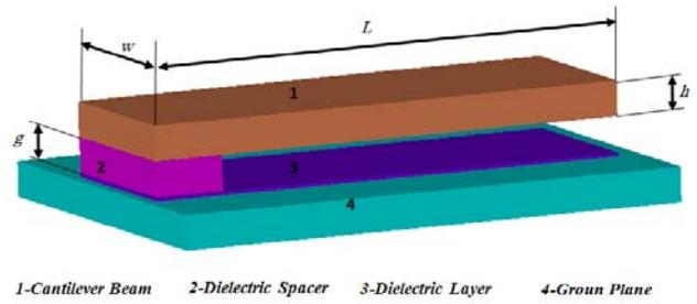
Fig. 1 Schematic representation of distributed model of micro cantilever-beam with a dielectric-layer
