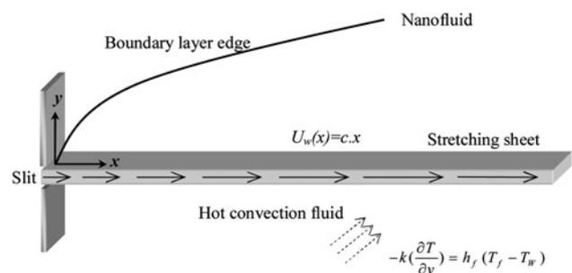
Fig. 1 Scheme of physical configuration of stretching sheet
