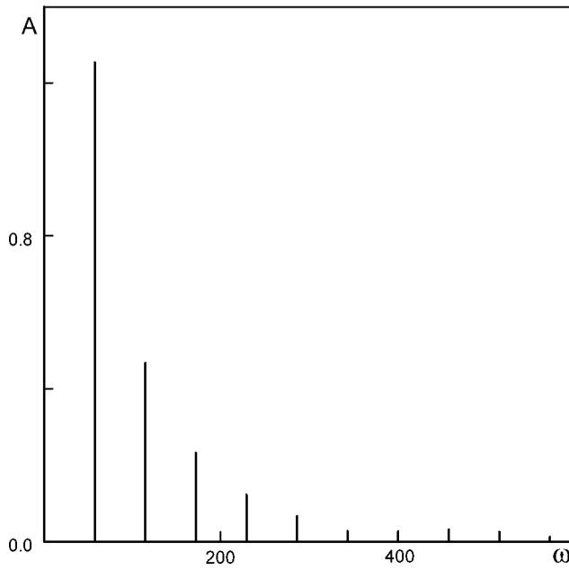
Figure 6. Eigenfrequencies of  $Nu$ , oscillation at  $Gr = 3 \times 10^5$ ,  $\alpha = 45^\circ$ ,  $f = 20\pi$ .
