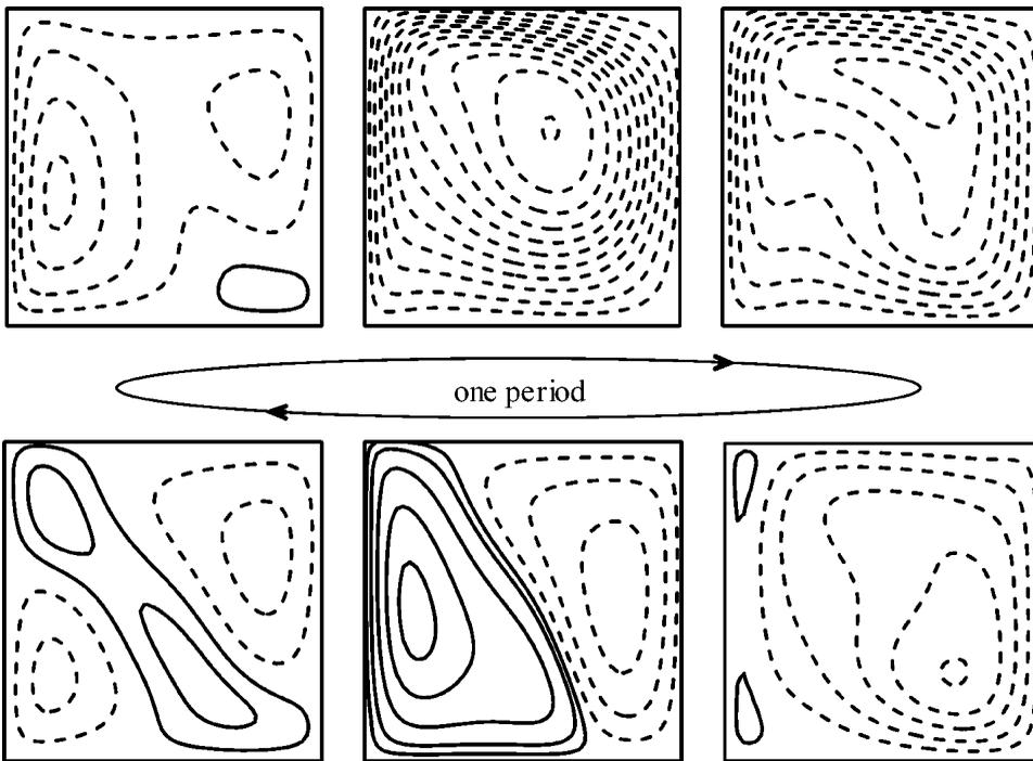
Figure 7. Representative plots of stream function (dashed lines correspond to negative values) during a period of oscillations.  $Gr = 3 \times 10^5$ ,  $f = 20\pi$ ,  $\alpha = 45^\circ$ .
