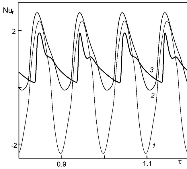
**Figure 2.** Heat flux  $Nu_r$  dependence on time for various values of  $\alpha$  at  $Gr = 2 \times 10^5$ ,  $f = 20\pi$ : 1,  $\alpha = 0^\circ$ ; 2,  $\alpha = 36^\circ$ ; 3,  $\alpha = 89^\circ$ .
