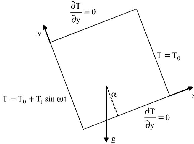
Figure 1. Enclosure geometry and temperature boundary conditions.
