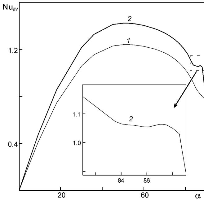
**Figure 9.** Time-averaged Nusselt numbers with inclination angle at  $Gr = 2 \times 10^5$  (1) and  $Gr = 3 \times 10^5$  (2) for  $f = 20\pi$ .
