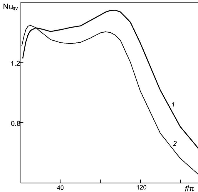
**Figure 10.** Time-averaged Nusselt numbers with frequency at  $\alpha = 50^\circ$  (1) and  $\alpha = 60^\circ$  (2) for  $Gr = 3 \times 10^5$ .
