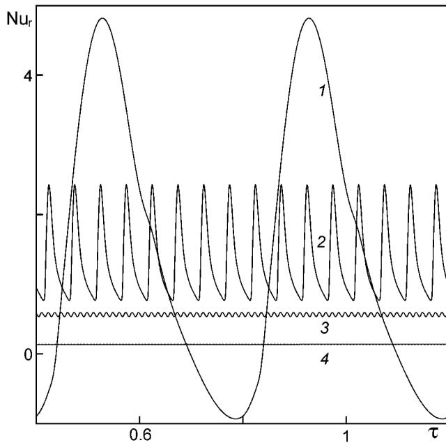
**Figure 4.** Heat flux  $Nu_r$  dependence on time at  $Gr = 3 \times 10^5$  and  $\alpha = 60^\circ$  for various values of  $f$ : 1,  $f = 5\pi$ ; 2,  $f = 40\pi$ ; 3,  $f = 160\pi$ ; 4,  $f = 320\pi$ .
