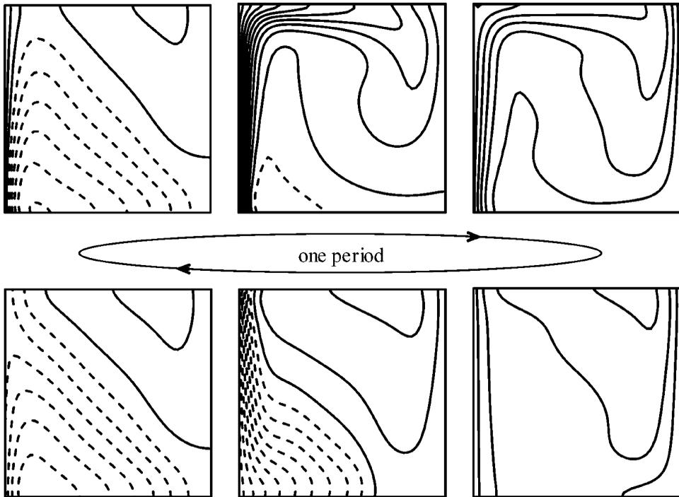
**Figure 8.** Representative plots of isotherms ( $\Delta\theta = 0.1$ , dashed lines correspond to negative values) during a period of oscillations.  $Gr = 3 \times 10^5$ ,  $f = 20\pi$ ,  $\alpha = 45^\circ$ .
